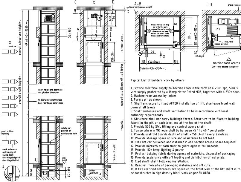
Ceiling below the lift shaft must support all strengths from the lift and must be calculated with a minimum of 5 kN/m2.
