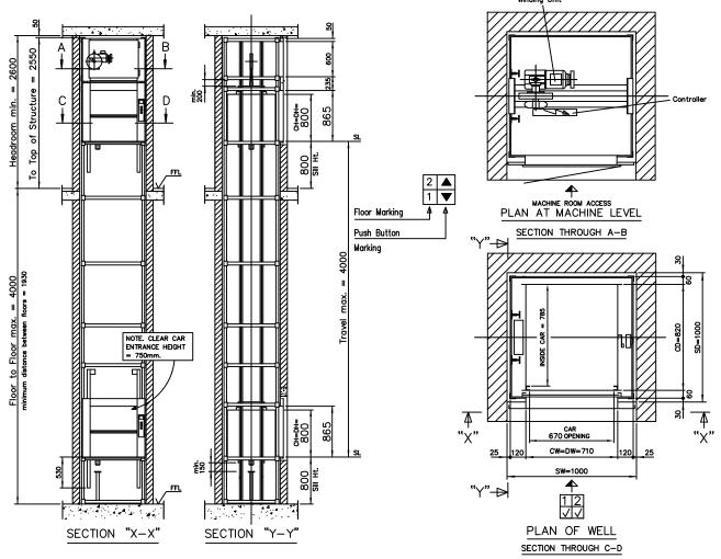
ERECTORS PLEASE NOTE! THIS LIFT IS SUITABLE FOR A MAXIMUM TRAVEL OF 4000MM, IF THE TRAVEL DIMENSION ON SITE IS LESS THAN 4000MM THE GUIDES/CORNER ANGLES MUST BE CUT TO THE CORRECT LENGTH PRIOR TO INSTALLATION.
